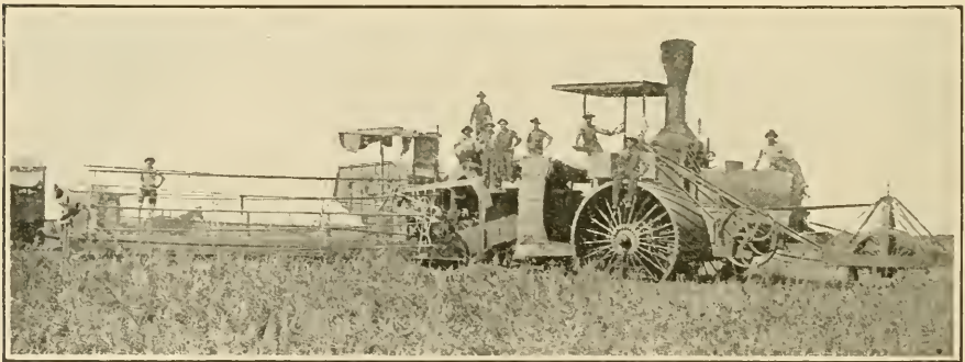
Best's Giant Combined Harvester and Thrasher. Will Cut, Thrash, and Sack the Grain at the Rate of 1,500 to 1,800 Sacks a day, and Covers an Area in That Time of One Hundred Acres
